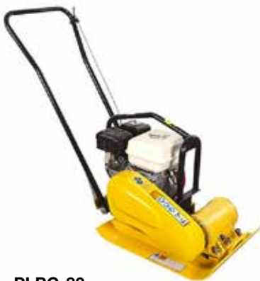
PLPC-80 Plate Size: 540x420mm Engine: PL-168F or Robin EY-20 Weight: 80Kg
