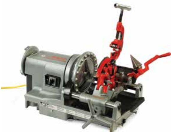
Model 300 Compact Capacity 1/4" - 2"
