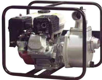
SEH-50X 2" (50mm) 30m Head, 600L/min Honda GX-120
