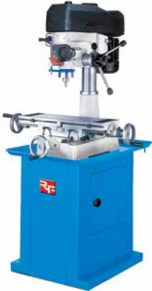
RF-25 Voltage: 230V, 1PH Drilling Capacity: 25mm (1") Face Mill: 76mm (3") End Mill: 20mm (3/4") Tapping: 16mm (5/8")
