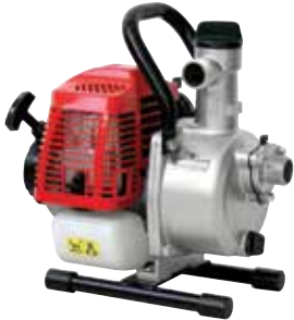
SEM-25L 1" (25mm) 35m Head, 115L/min Mitsubishi TU-26
