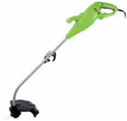
PLGT-1000 Power: 1000W String Spool: 2.0mm x 5m Cutting Width: 350mm
