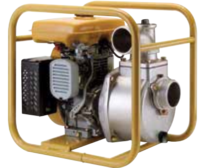
SE-50X 2" (50mm) 30m Head, 600L/min Robin EY-15
