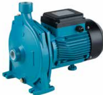
PLCP-158 / PLCP-400 / PLCP-500 Power: 1 / 1.5 / 2.0HP Head: 32 / 40 / 45m Flow Rate: 110 / 120 / 150L/min
