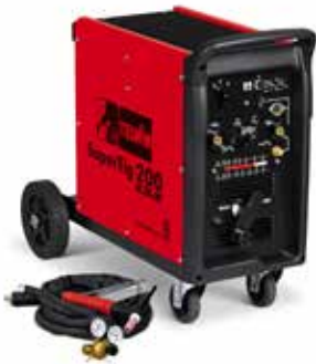
Supertig 200 AC/DC-HF For welding aluminium and all other types of materials
